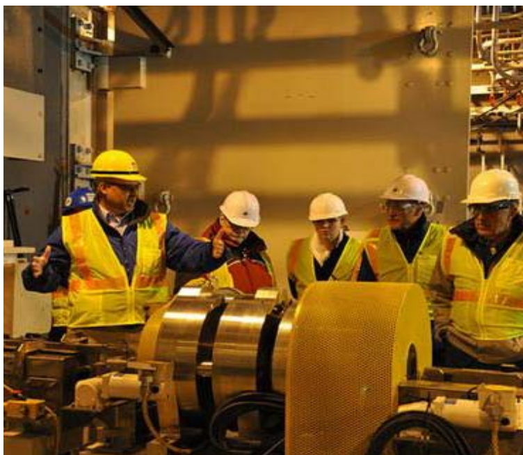
A team from the Centers for Disease Control and Prevention (CDC), Atlanta, Ga., listens as Blue Grass Chemical Agent-Destruction Pilot Plant Chief Scientist Dr. John Barton details how the Rocket Cutting Machine separates rocket warheads from their motors and transfers the warheads for subsequent agent draining.
